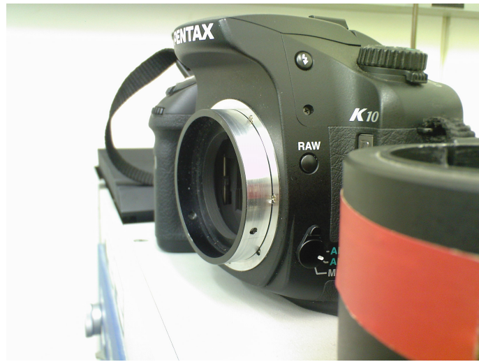
fig. 2: Mounting of my camera on the used microscope
